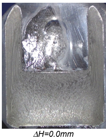
Figure 9: Cross-sections showing the grain flow during forming
