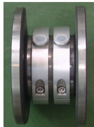
Figure 4: Load cell with strain rings attached
